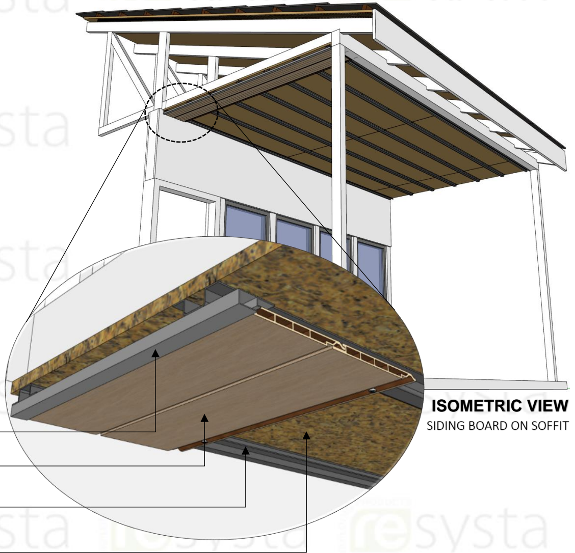
ISOMETRIC DETAIL SIDING BOARD ON SOFFIT
