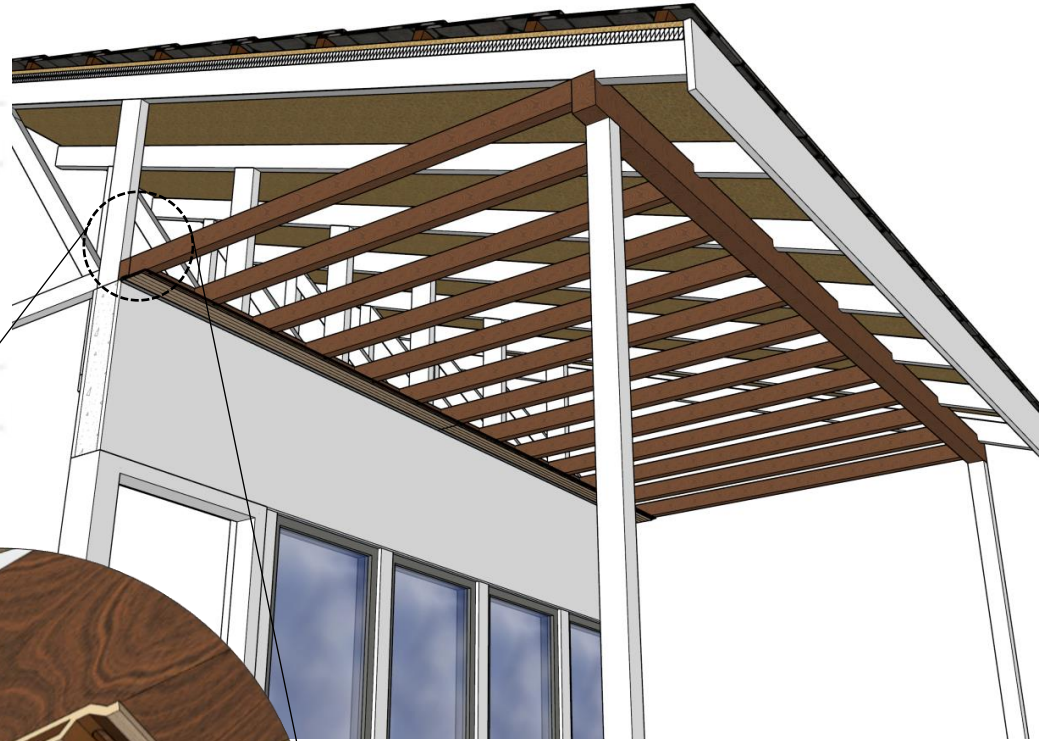
ISOMETRIC VIEW SIDING BOARD ON SOFFIT
