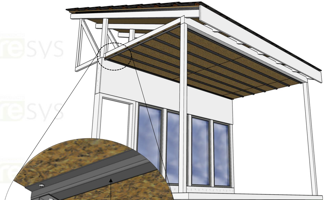
ISOMETRIC VIEW STARTER STRIP AND J-MOLD
