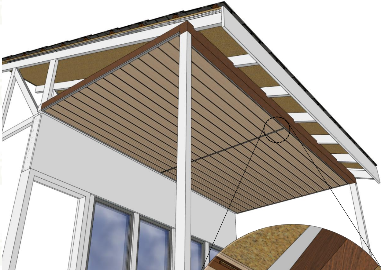
ISOMETRIC VIEW SIDING H-MOLD
